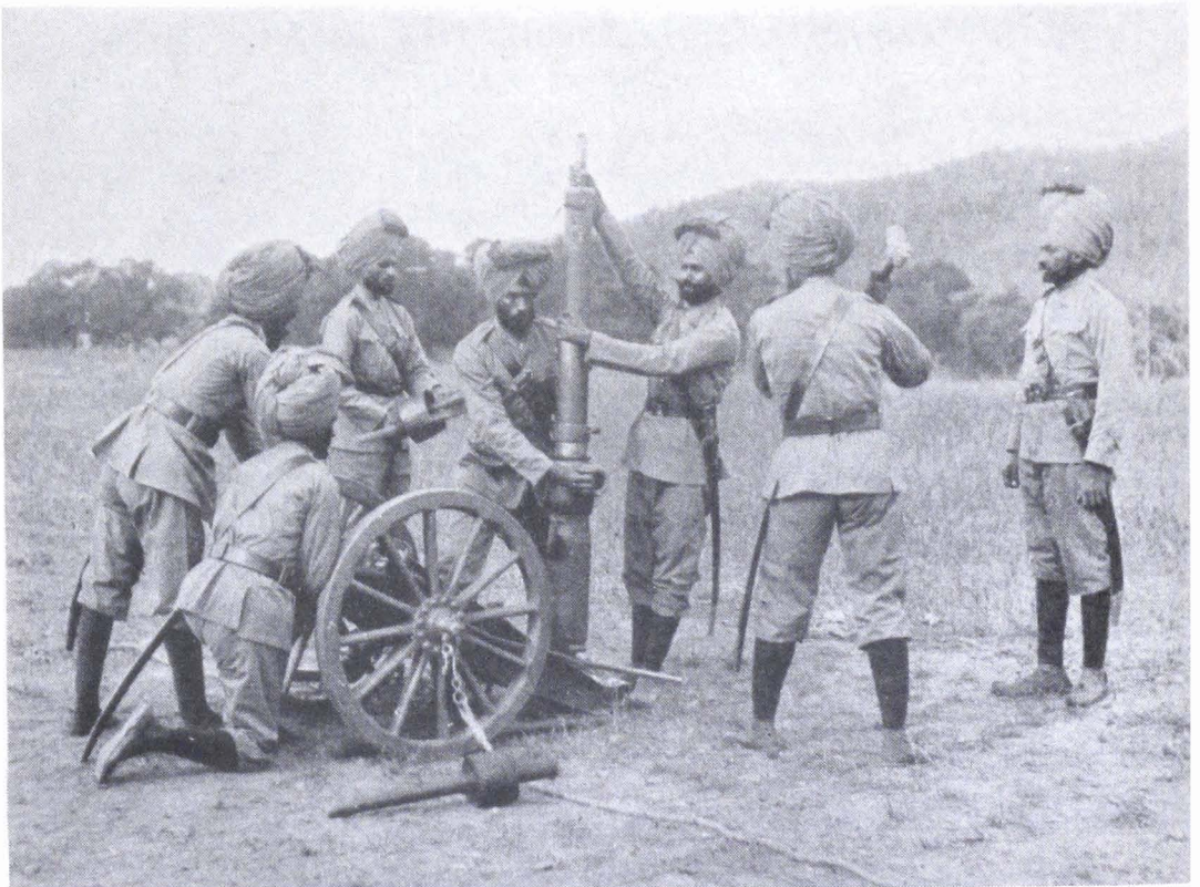
Assembling the 2.5-inch M.L. Gun: The Screw Gun
